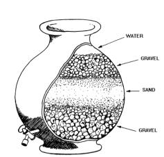
Figure 2: Small-scale sand filter
